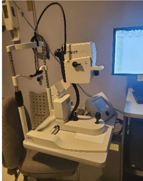
Figure 2. The Heidelberg Spectralis was used at each imaging session to acquire radial OCT image volumes consisting of 24 slices per volume
