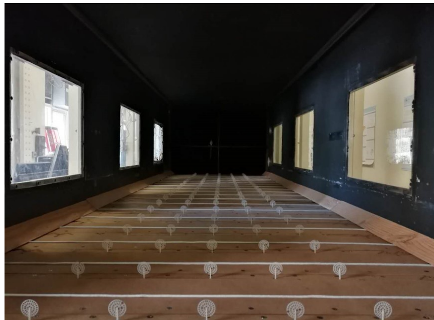
Figure 4 Photograph of the roughness elements applied to the micro wind farm in the wind tunnel
