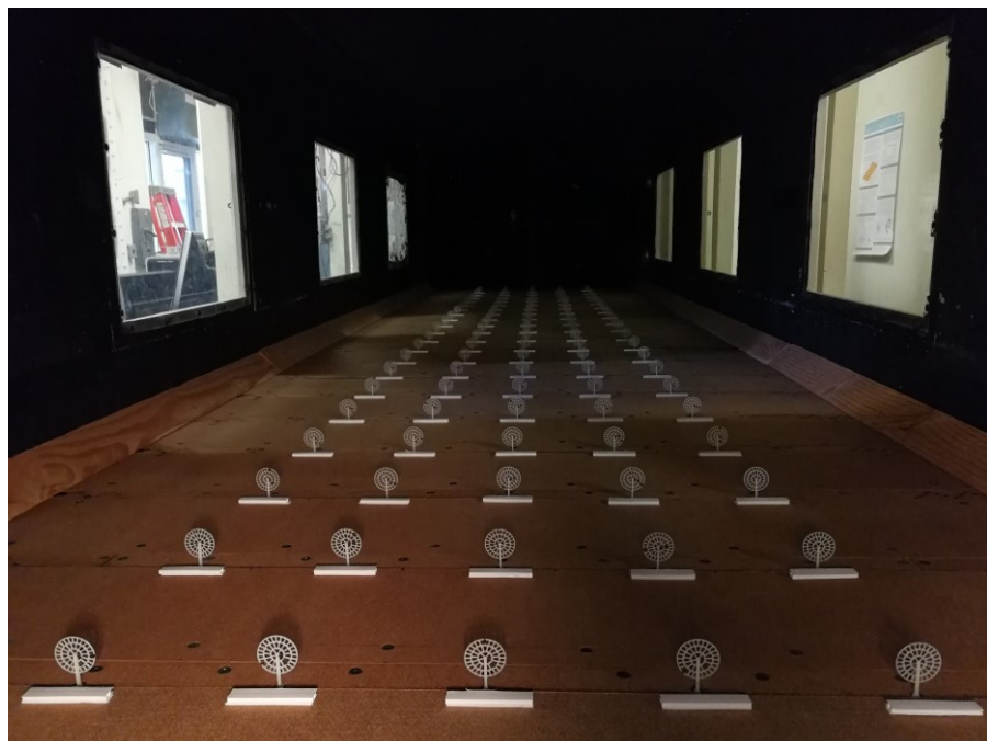
Figure 8 Overview photograph of windbreaks applied to micro wind farm in the
