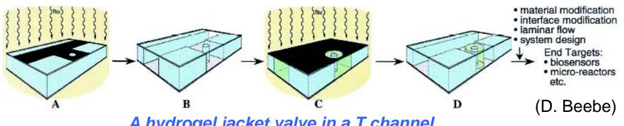
A hydrogel jacket valve in a T channel
