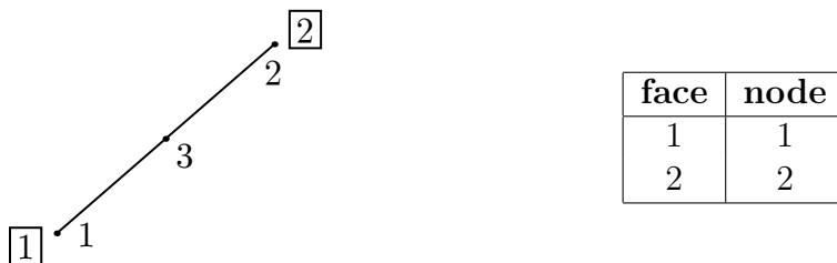
Figure 7.1: Node, face, and node-on-face numbering for line integration domains.
