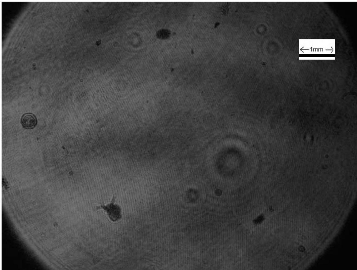
Original size is 2832x2128, Grayscale. In the lower left corner is a Daphnia, also known as a “water flea”. I reconstructed the image in depth from 0-15mm in increments of 250 microns. See **Appendix A** for specific camera settings and program data entries.
