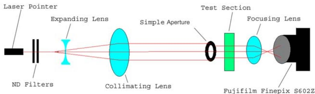
The beam source is a \$10 laser pointer by "Lazerpro". The batteries ran out on the first day so after that it was connected to a variable power supply set at 4.5v.
