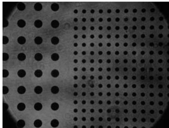
As you can see, the field of view is the same in both images, so the smaller resolution image still uses the whole CCD chip and just drops pixels (meaning the pixel spacing is much larger!).
