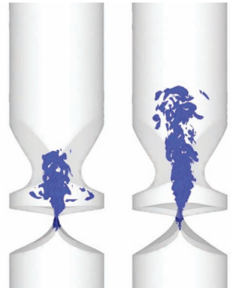
Fig. 3. Computer simulation of phonation for a simplified model based on a CT scan. Figure shows formation of the glottal jet.
